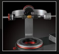
**BULLET HOLDER** Universal bullet holder for 360° bullet rotation of pristine or damaged bullets
