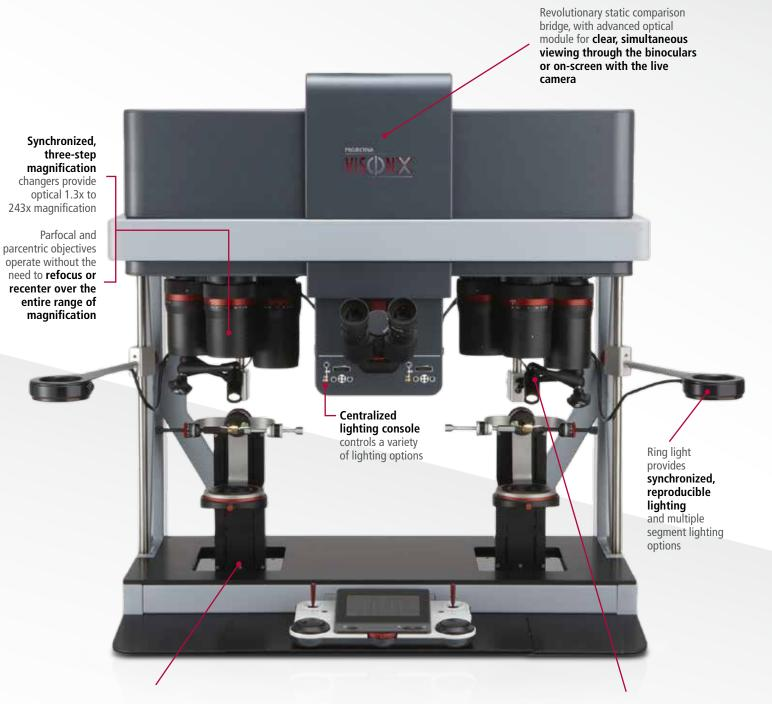
**Motorized stages** with 50 mm (2 in.) of X/Y movement and a height adjustment of up to 146 mm (5.8 in.)
