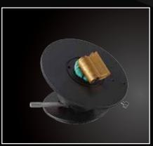
BALL-MOUNTED ROTATING/ TILTING STAGE Rotating and tilting ball-mounted platform for larger objects and toolmarks
